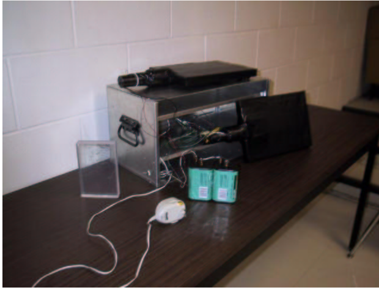
Figure 4: Above all of the components of the C.R.D. have been removed from the aluminum box for better viewing. The batteries and DC adapter are the power supply options.
