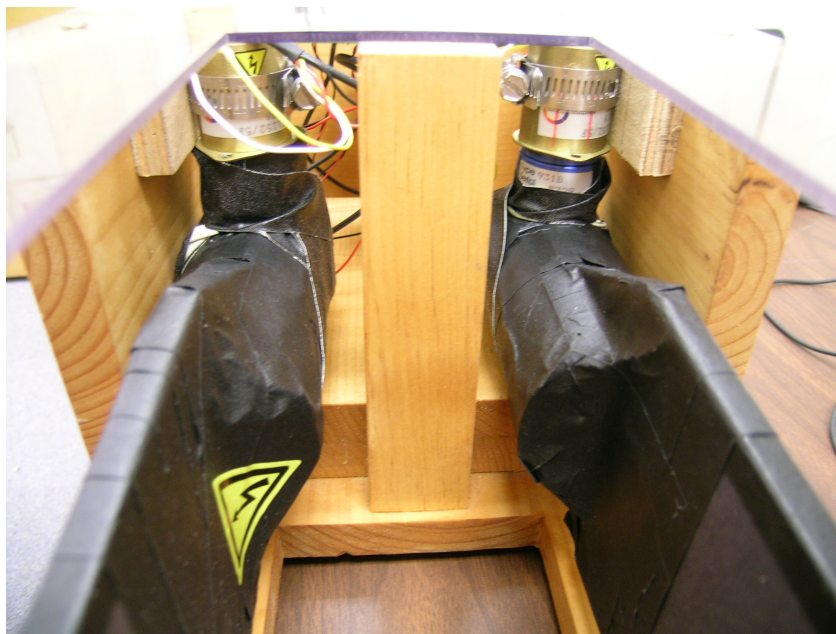
Figure 19: Sidemount photomultipliers attached to scintillators.
