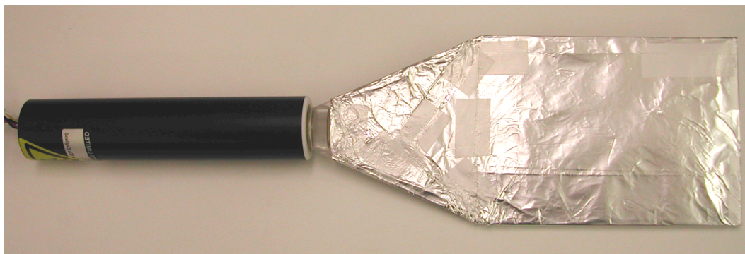
Figure 10: Scintillator paddle wrapped with aluminum foil.
